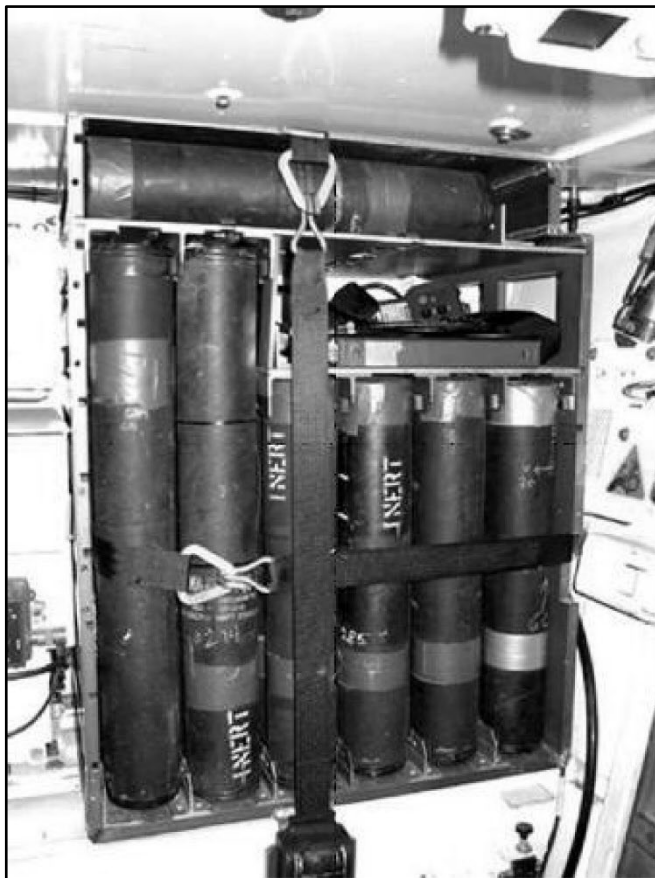
Figure 5-31. Right side ammunition rack
