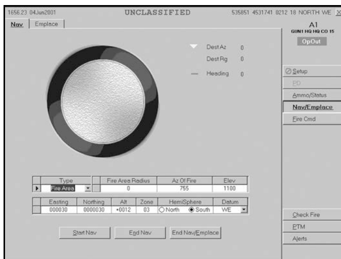
Figure 6-21. Navigation/emplacement screen: fire area
