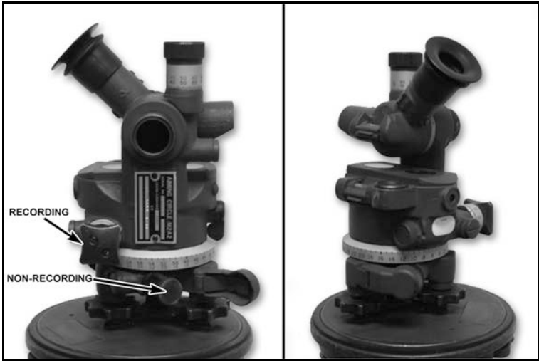
Figure 3-15. Aiming circle, M2A2
